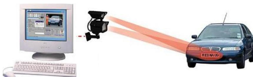
**Fig. 1. Hardware and software components of ANPR system**
