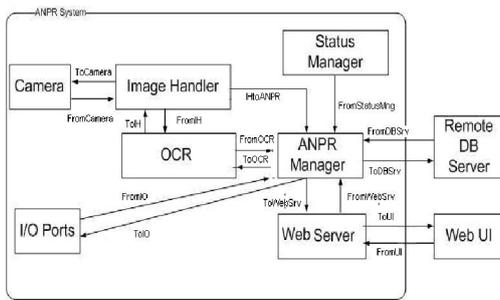
**Fig. 3. CSP processes of ANPR System**
